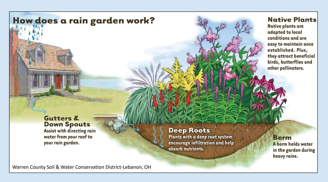
Rain gardens are shallow basins planted with native vegetation that are used to manage stormwater. When stormwater runoff from a paved parking lot, rooftop, or a compacted lawn flows into a rain garden, the water slowly soaks into the soil and replenishes groundwater, instead of flowing into the storm drain. Rain gardens capture and store stormwater before it becomes polluted by fertilizer, road salt, motor oil, and other pollutants, helping to keep the Wallkill River clean.
